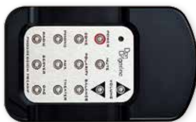
ABOVE: As supplied with the Progression preamp [HFN Apr '18], this chunky BT remote offers volume, balance, mute, polarity and (analogue) input selection
